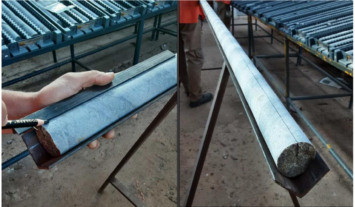
Figure 10-9: Drill Core Orientation Process
