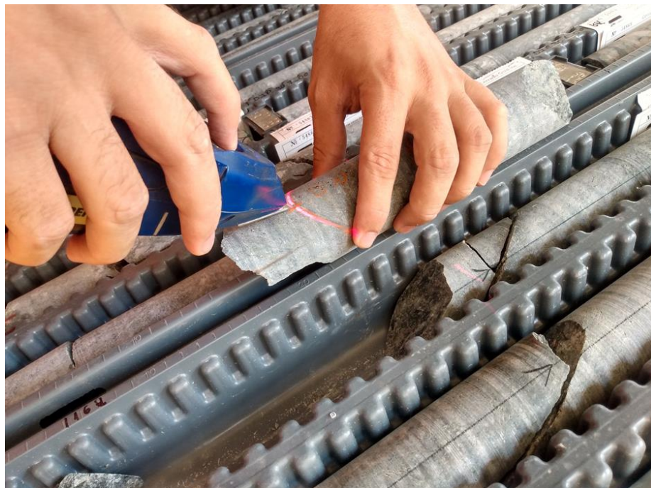
Figure 10-10: Process of Collecting Structural Data on Drill Core
