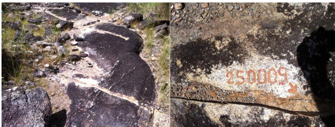
Figure 9-15: Kinross Channel Samples Collected in Hard Rock Using Electric Saw with Diamond Blade
