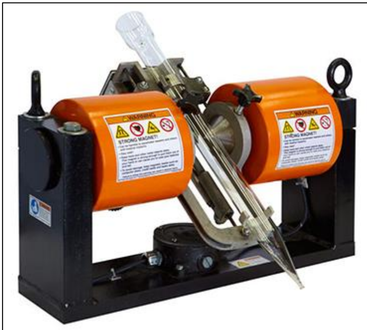
Figure 11-1: A Davis Tube magnetic separator
