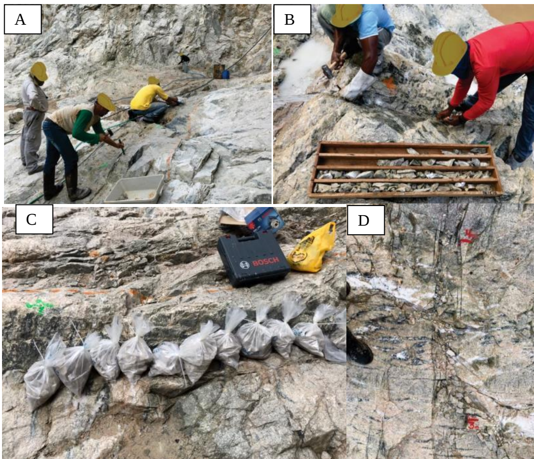
Figure 9.21 MSM Channel Sampling
