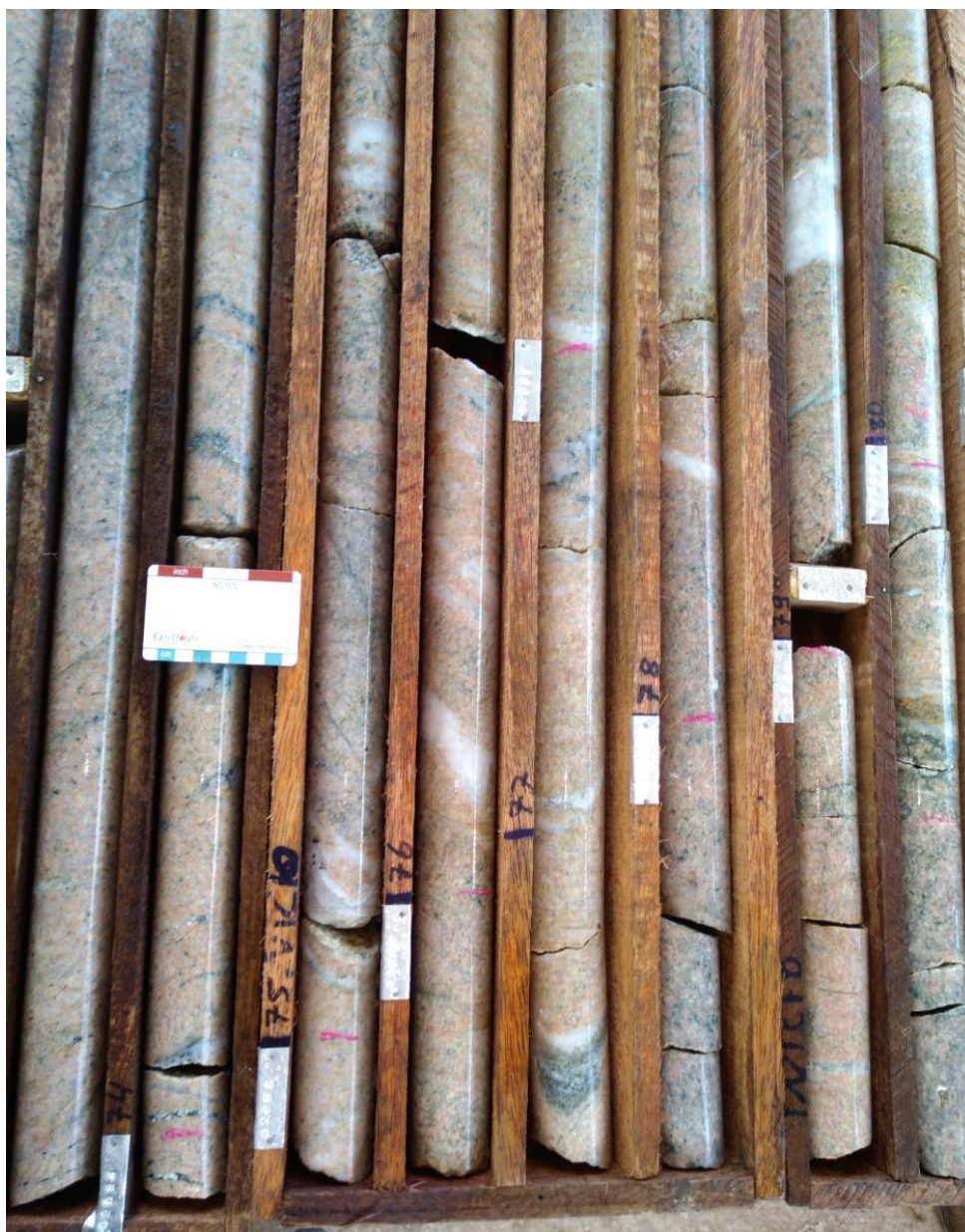
Figure 10.6 Mineralized and Altered Granite Showing Good Recovery
