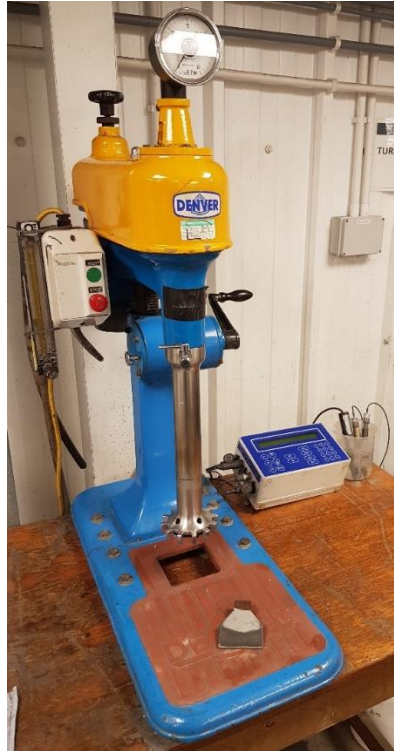
Figure 13-5 - Denver D12 laboratory flotation machine
