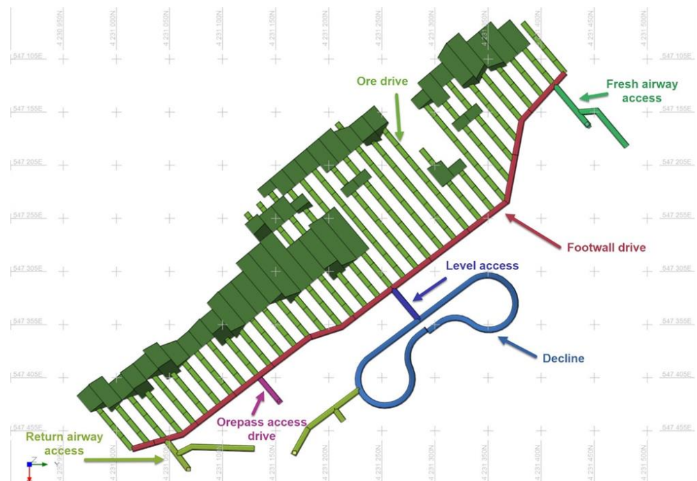
Figure 16-27 – Typical level layout (plan view – 220 South Level)
