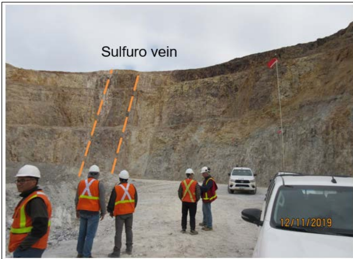
Figure 14.2: Well Defined Sulfuro Vein Defining High-Grade Wireframe
