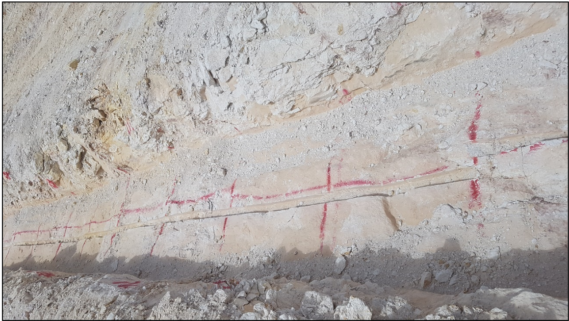
Figure 10.3: Typical Trench Sampling at Martinetas
