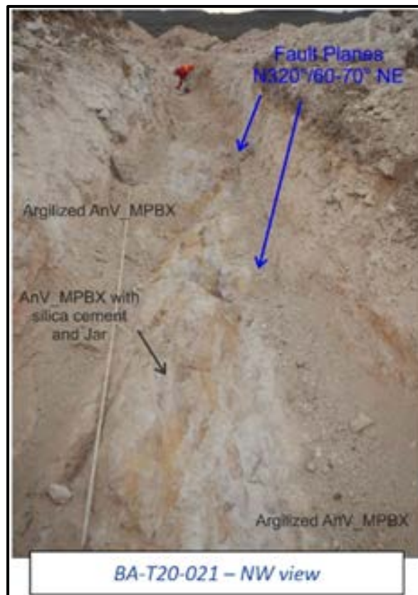
Figure 9.2: Fault Cutting Baritina Breccia Pipe Exposed in Trench
