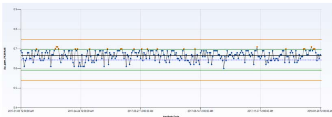
Figure 11.3: Shewhart Control Chart for Standard GS-P5D for 2017
