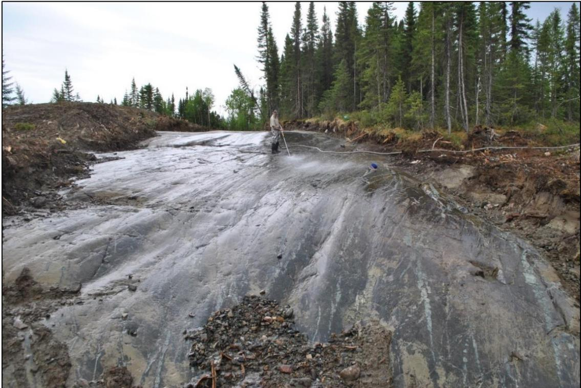
**Figure 9-1 – Washing of a stripped area on the South Zone**
